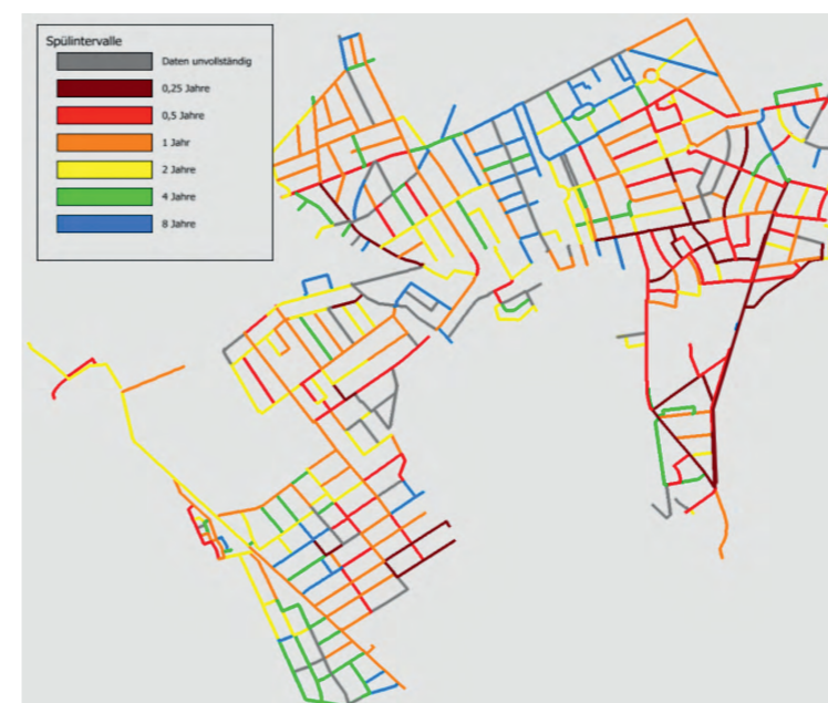
Evaluation of flushing data with conduction of flushing intervalls
